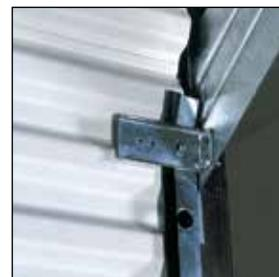
12-gauge, zinc-coated door stops are mounted to brackets for increased strength. 18-gauge, zinc-coated steel guides with polypropylene runners allow doors to glide smoothly.
