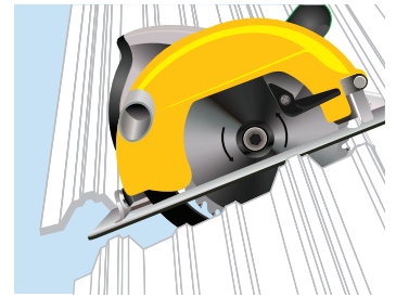
Sawing the panels Figure 4
