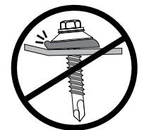
INCORRECT Non-perpendicular. Figure 8c
